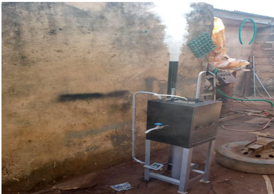
Fig. 1. Pictorial View of the Fabricated Refuse Fired Boiler
